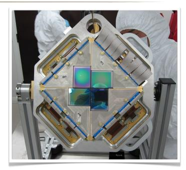
450 µm focal plane unit prior to installation
